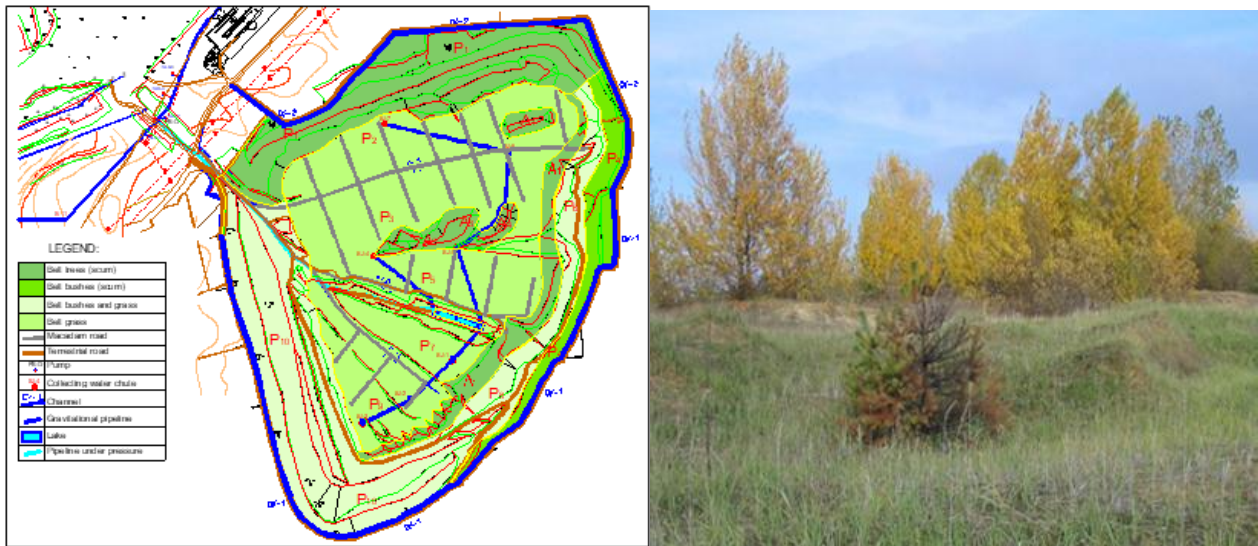
Figure 4: Final rehabilitation phase of the external dump
