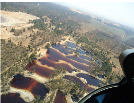
Fig. 11: Acid mine water above a collapsed room-and-pillar coal mine, province Mpumalanga, South Africa (Henk Coetzee, Geological Survey of South Africa)
