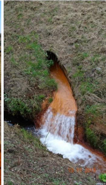
Fig. 9: Mine water with high content of Iron 2+ coming to the surface (own picture)
