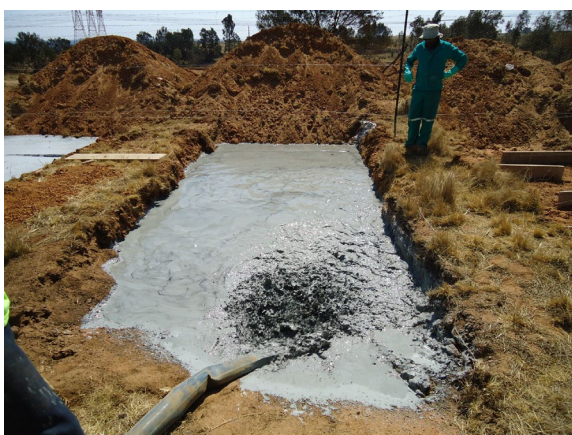
Fig. 29: Test field with a slurry with fly ashes from power plants (Henk Coetzee, Geological Survey of South Africa)
