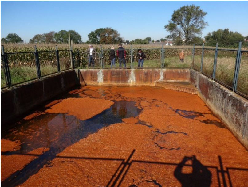
Fig. 9: Mine water with high content of Iron 2+ coming to the surface (own picture)
